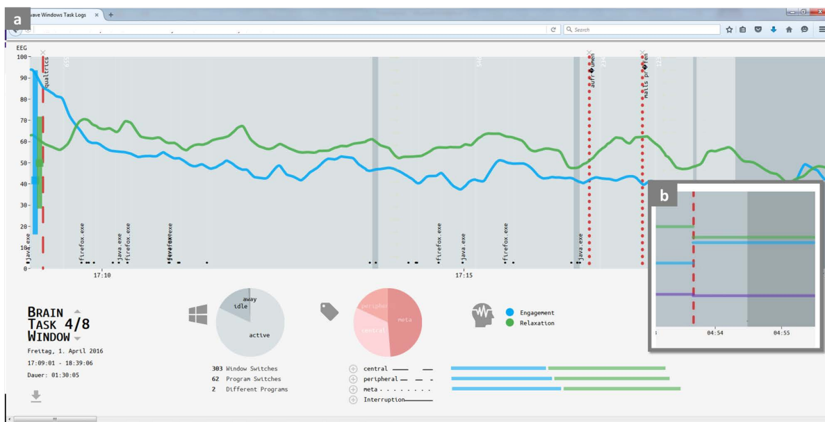
Figure 1. (a) Session view showing EEG Engagement (blue), relaxation (green) as a line graph. Working spheres are depicted using dashed lines, PC activity depicted using grayscales. Summary of window and task activity is shown as pie charts. Names of tabs, programs and tasks are written vertically on the top graph. (b) Average engagement and relaxation scores per task view shown when users click on the corresponding signal type.
