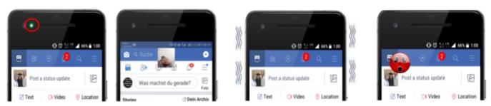
Figure 3. DSSytem interface in case of shoulder surfing: LED flash light is on(Left), a preview of the front camera appears (second to left), vibration(second to right) and icon overlay (right)
